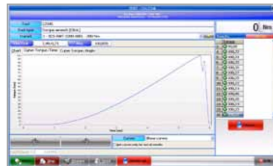
Torque\Time Curve: AWT detects the click point
