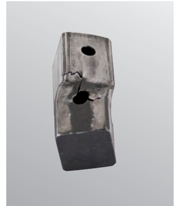
OTHERS: Uncontrolled breakaway can damage other components
