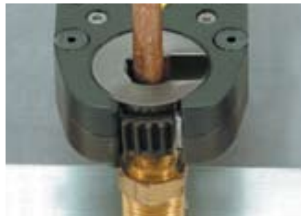
Slide the tool on the fastener and push the throttle lever down fully to run the fastener down.
