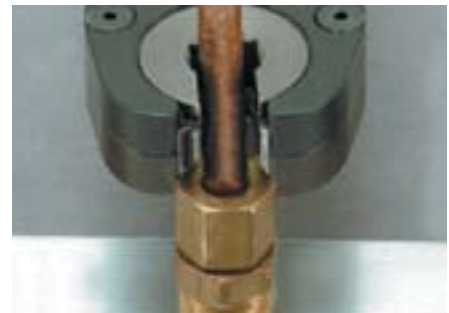
To free the tool, slide the tool off the tightened fastener and operate the throttle lever halfway to release the socket back to the open position.
